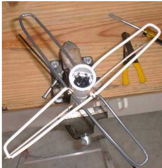
Figure 4: 70 cm beam feedpoint arrangement inside a PVC coupling.
